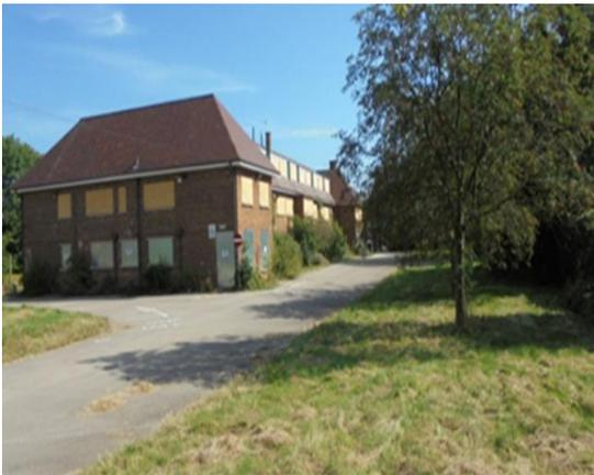
The building comprised of brick & concrete construction (two storey) with solid brick and studded partition walls. Roof construction was a timber pitched roof with tiled cladding. There was a basement void beneath ground floor slab.
